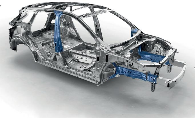
A double-ring structure provides the bodyshell with a naturally strong frame, in particular reinforcing the rear of the car and the area around the tailgate
